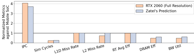
Fig. 11. RTX 2060 architecture's performance improvement over Mobile SoC
